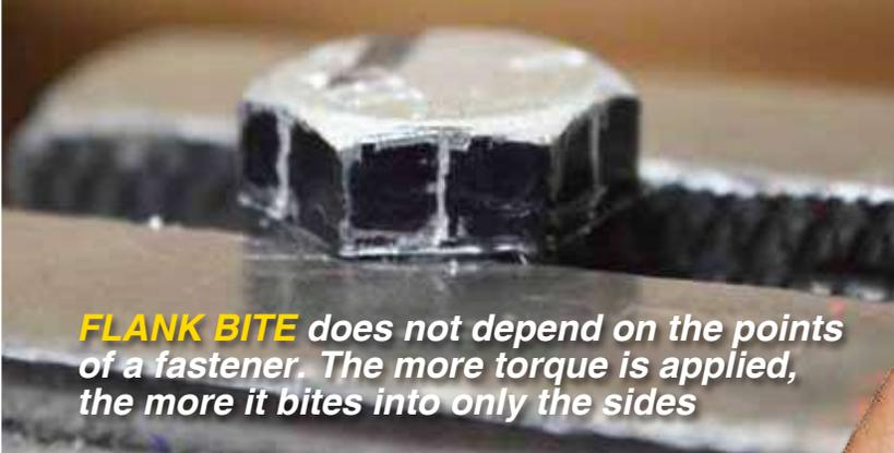
**FLANK BITE** does not depend on the points of a fastener. The more torque is applied, the more it bites into only the sides
