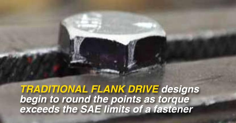
**TRADITIONAL FLANK DRIVE** designs begin to round the points as torque exceeds the SAE limits of a fastener
