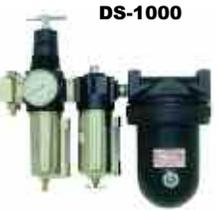
DS-1000                       | M-1000                                | System Supreme Desiccant Dryer System                                                                      | Supplies clean, ultra-dry, oil free air to the booth. A particulate filter, oil coalescer, desiccant dryer and regulator.                     | Pipe Size: 1/2NPT<br>Nominal Airflow: 30 CFM<br>Filtration Rating: .01 Micron<br>Max. Pressure: 125 PSI<br>Max. Temp.: 120F  |
