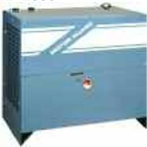
RF-2050                         | RF-2055                               | Refrigerated Dryer                                                                                         | Removes moisture from compressor discharge by lowering temperature. An efficient and economical way of providing dry air throughout the shop. | Nominal Airflow: 20 CFM<br>Comp. Rating: 5 HP<br>Inlet Temp.: 100F<br>Voltage: 115/220V 1Ø                                   |
